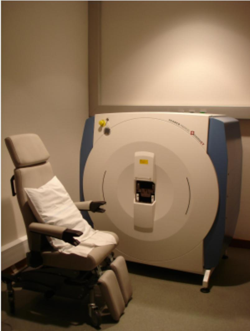
**The XtremeCT is a high resolution peripheral CT for human in vivo measurements of both bone density and bone microarchitecture.**
